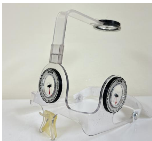
Rycina 10. Cervical Range-of-Motion instrument
